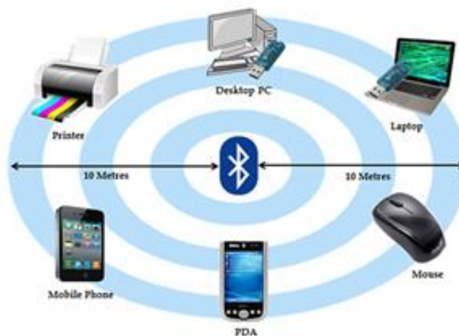
Figure 10: Multiple devices Bluetooth connection
